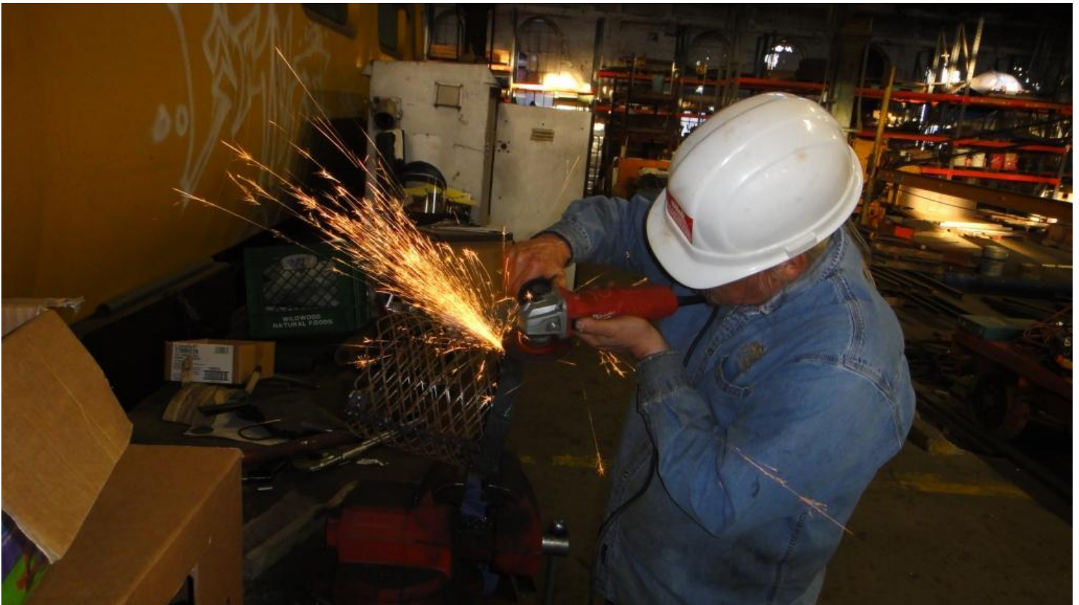
Fred grinds-off rough edges on a new shield.
