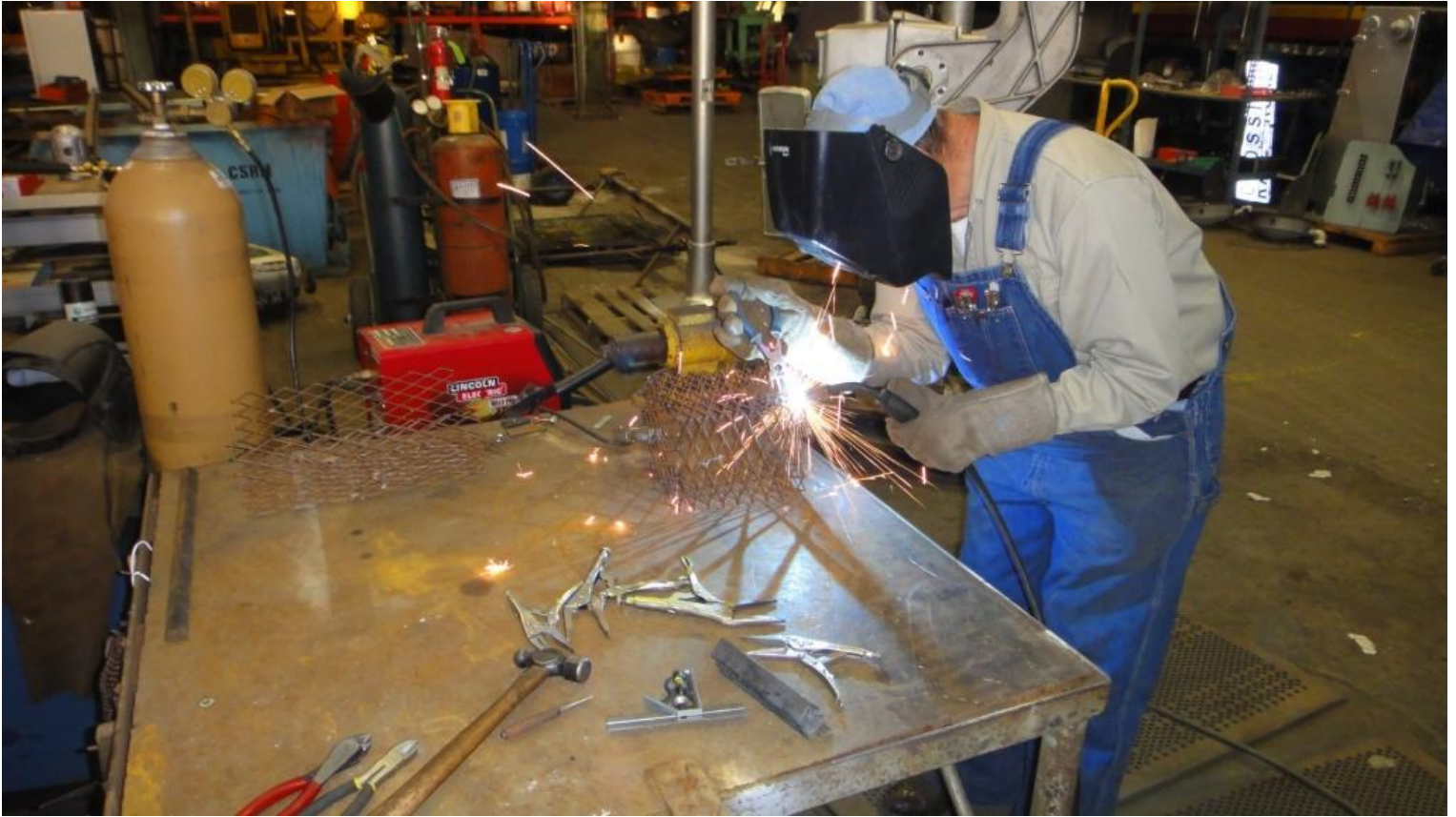
Cliff welds a protective shield together
